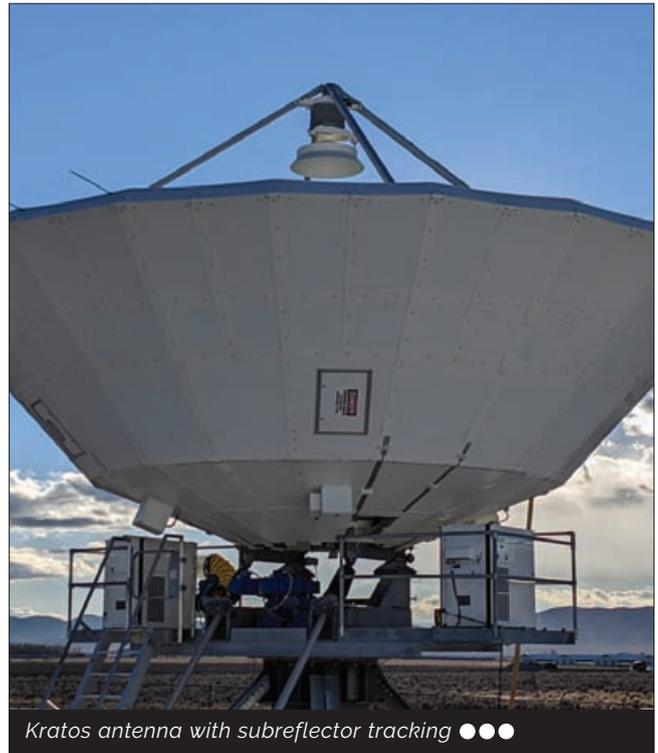
Kratos antenna with subreflector tracking ●●●
