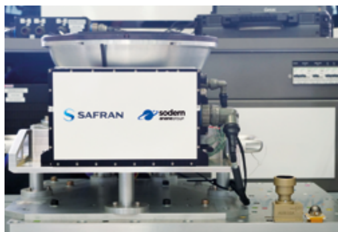
PROTOTYPE TEST OF DAYLIGHT STAR TRACKER ON A 4X4 VEHICLE
