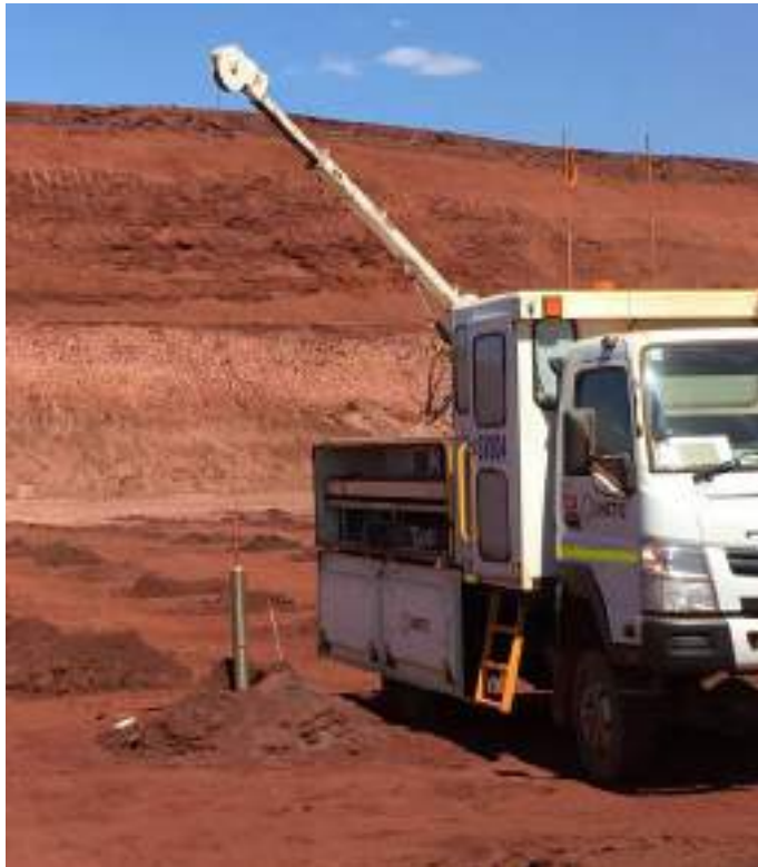
Open-pit blast hole logging with FastGrade™
